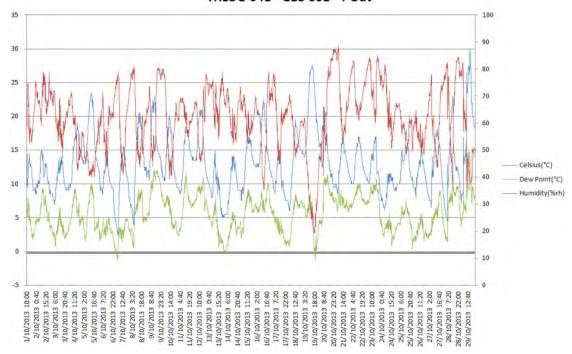
Figure 2: Example of graphed raw data from temperature/humidity data loggers
