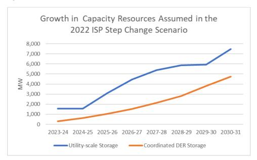
As Figure 1 demonstrates, the ISP assumes both utility-scale and coordinated DER storage will grow significantly this decade, with utility-scale storage increasing by 6 GW at an average, annual rate of growth of 28%, while coordinated DER storage is assumed to increase by 4.4 GW at an average, annual rate of growth of 49%.<sup>5</sup>
