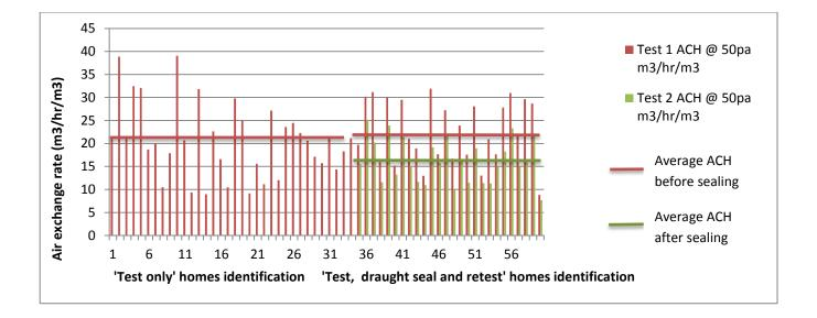
Figure 40: Air exchange rates of 60 homes before draught sealing and at 26 of these homes after draught sealing, noting average air exchange rates/hr are 28% less after draught sealing
