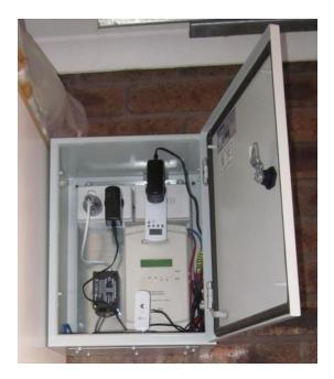
Figure 6: Remote enclosure with Ecofront and communications equipment
