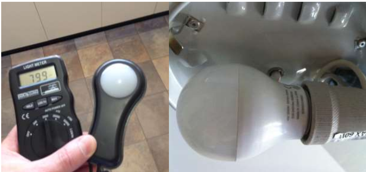
Figure 4.64 a) Light meter used to assist participants in understanding the improvement in light levels from retrofits; b) LED globe retrofit.
