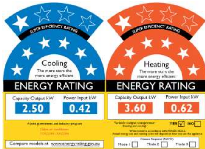
Figure 4.62 An energy rating label from one of the reverse cycle air conditioning retrofits of this project.
