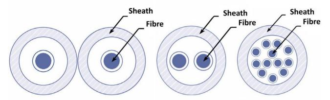
*Security Control: 0190; Revision: 2; Updated: Sep-18; Applicability: O, P, S, TS; Priority: Must If a fibre-optic cable contains subunits, each subunit only carries a single group; however, each subunit in the cable can carry a different group.*
