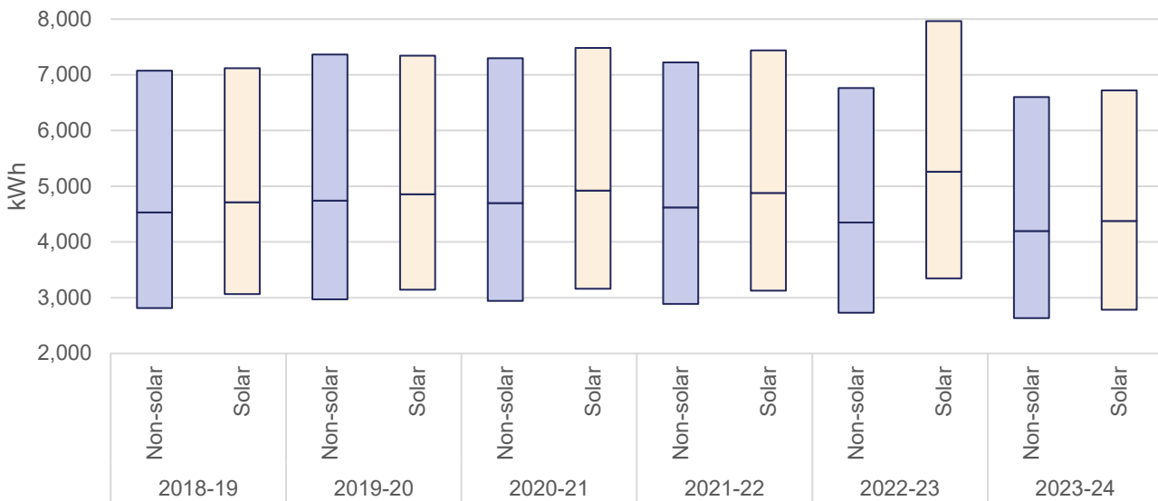
Figure 3: Annual grid use by residential households with and without solar – 25 th , median and 75 th percentile
