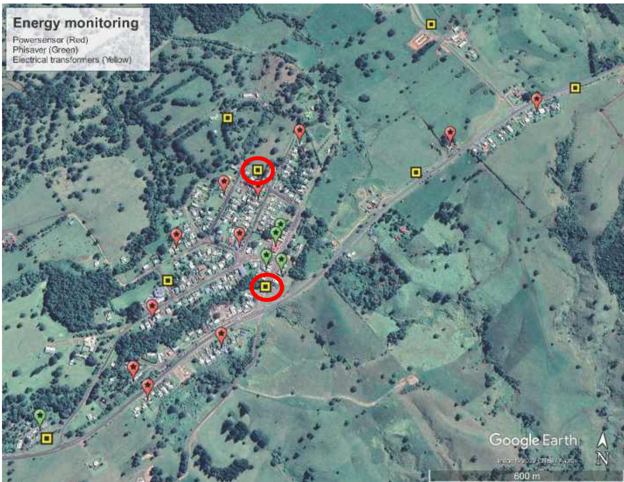
Figure 7: Location of SS10112 and SS1256 transformers (denoted by red circles around the yellow transformers). This figure is an adaptation of Figure 3 above
