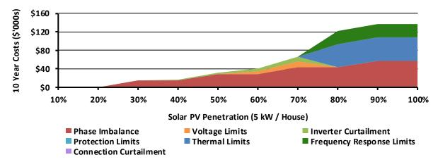
Illustration of Overhead, Urban LV Network Integration Solution Costs by Inverter Penetration Level
