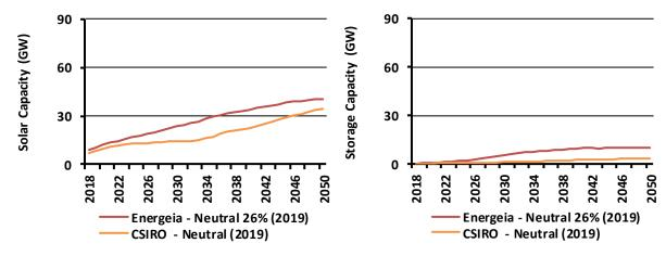
Figure 6 – Rooftop Solar PV (Left) and Behind the Meter Storage (Right) Uptake (GW) Forecasts
