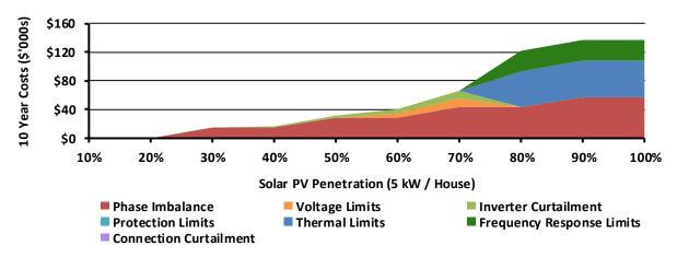
Figure 28 – Illustration of Network Integration Solution Costs by Inverter Penetration Level
