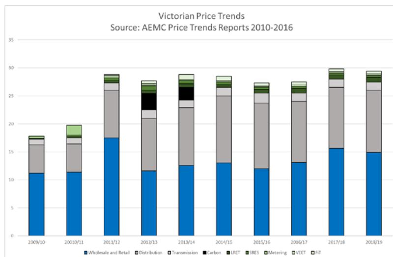
Figure 4 simplifies this chart by grouping network costs together, the environmental costs together and comparing these to the AEMO wholesale electricity price. This chart more clearly shows that the network component in Victoria has driven price increases from 2009 to 2014, and that the combined 'competitive market' elements are expected to drive increases beyond 2016.
